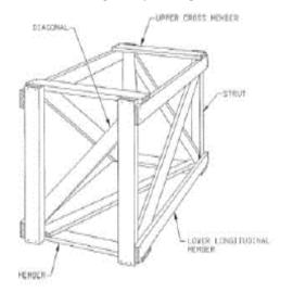
Left: Crate designs should make use of diagonal members to increase the structures rigidity. Please use screws as fasteners. This will allow our associates to easily remove the crate when needed without damaging the products.
